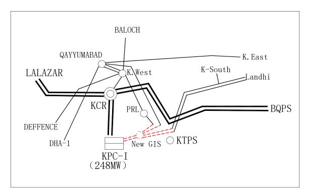
Fig.4.2-1 Alteration Scheme Sketch of KPC-I Evacuation System
