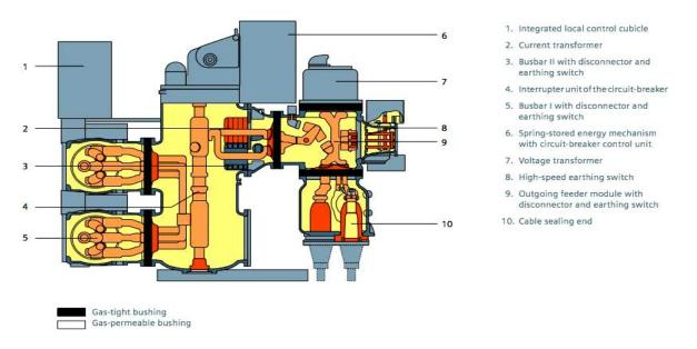
Figure 6: Schematic Representation of a Typical GIS
