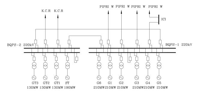
Fig. 4.1-1 Existing Electrical Single Line Diagram of BQPS Power Plant
