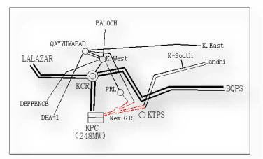
Figure 9: The Existing Evacuation System of KPC
