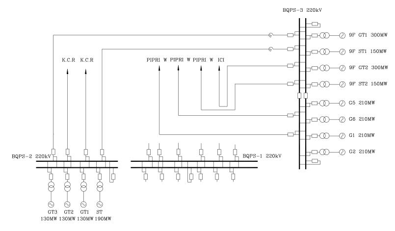
Fig 2.8-3 The SLD of 220 kV GIS with 2<sup>nd</sup> 9F Combined Cycle in Phase three
