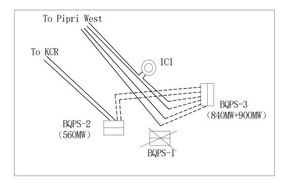
Fig.4.4-1 Interconnection Scheme Sketch of BQPS-3
