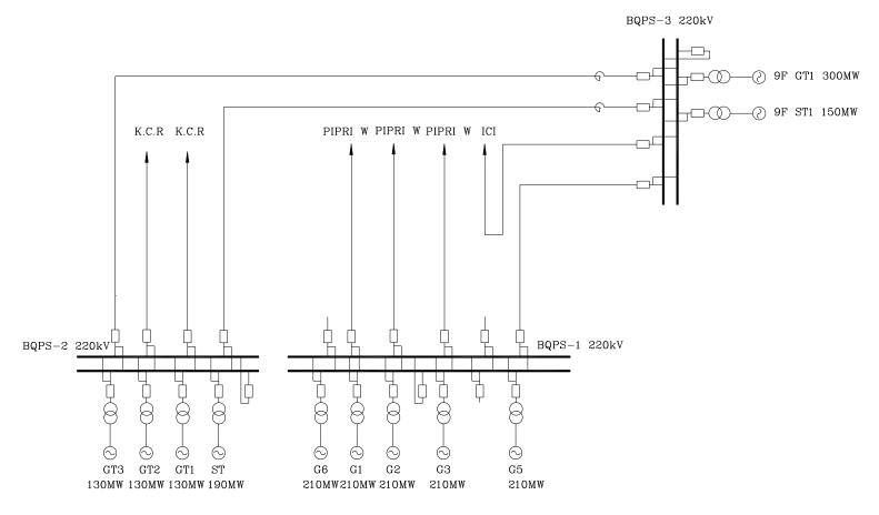
Fig 2.8-2 The SLD of 220 kV GIS with 1<sup>st</sup> 9F Combined Cycle in Phase two
