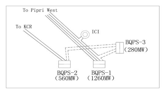
Fig.5.2-10 Temporary Interconnection Scheme Sketch of BQPS-3 (Single Bus)
