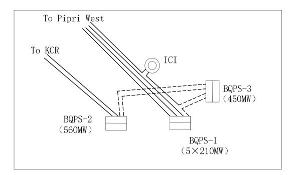
Fig.4.4-3 Temporary Interconnection Scheme Sketch of BQPS-3
