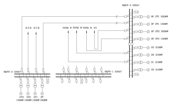
Fig.4.4-2 Final Electrical Single Line Diagram of BQPS
