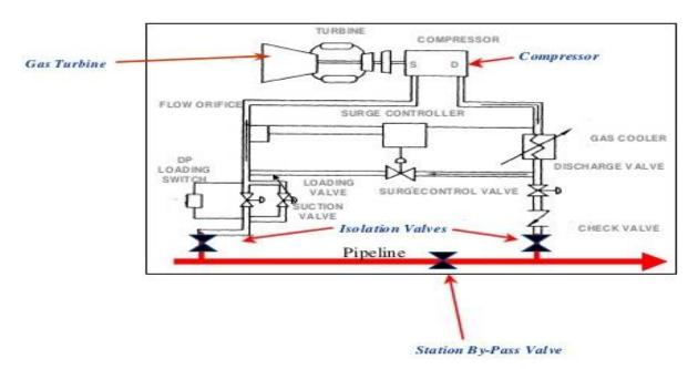
Figure 8: Schematic for Typical Gas Compressor Station
