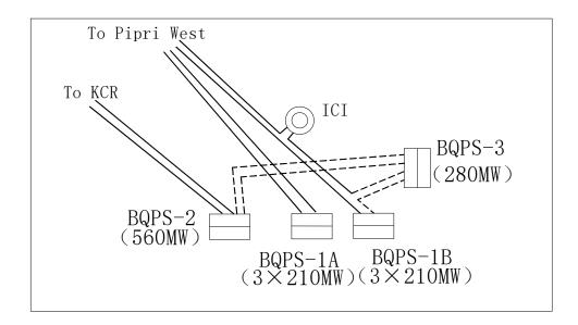
Fig.5.2-10 Temporary Interconnection Scheme Sketch of BQPS-3 (Split Bus)
