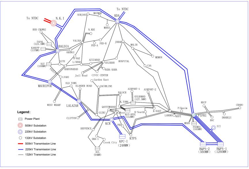
Fig .2.1-1 Network Diagram for Karachi 132kV and above Grid in 2016
