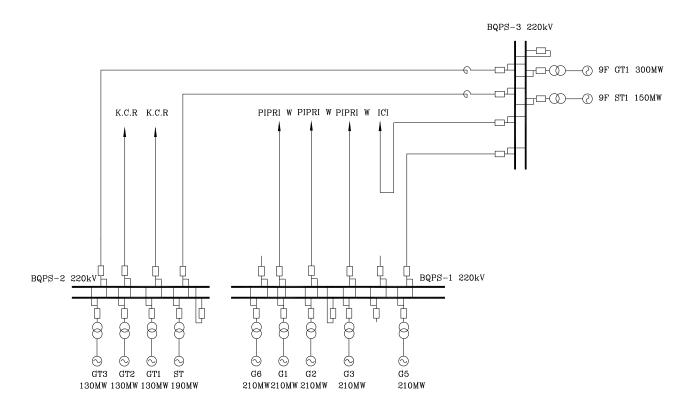
Fig.4.4-4 Electrical Single Line Diagram of BQPS during Construction Period
