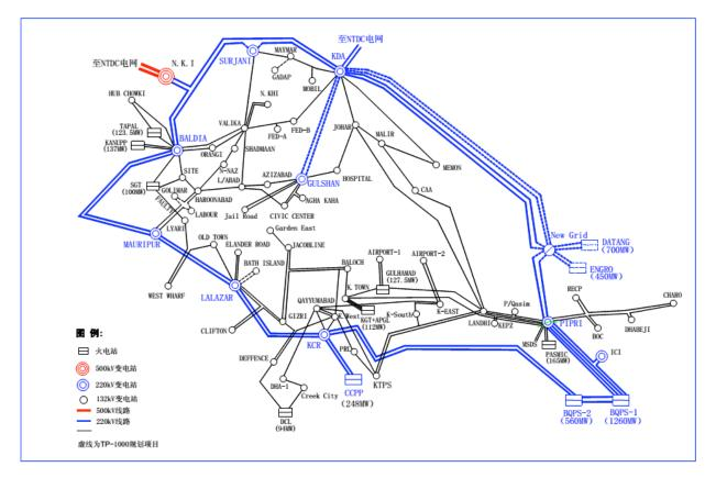
Fig. 2.3-1 Planned Grids Map above 132 kV of Karachi Power System in 2020.
