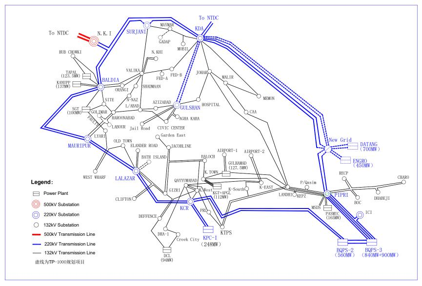
Fig.4.3-1 Network Diagram for 132kV and 220kV Grid in 2020
