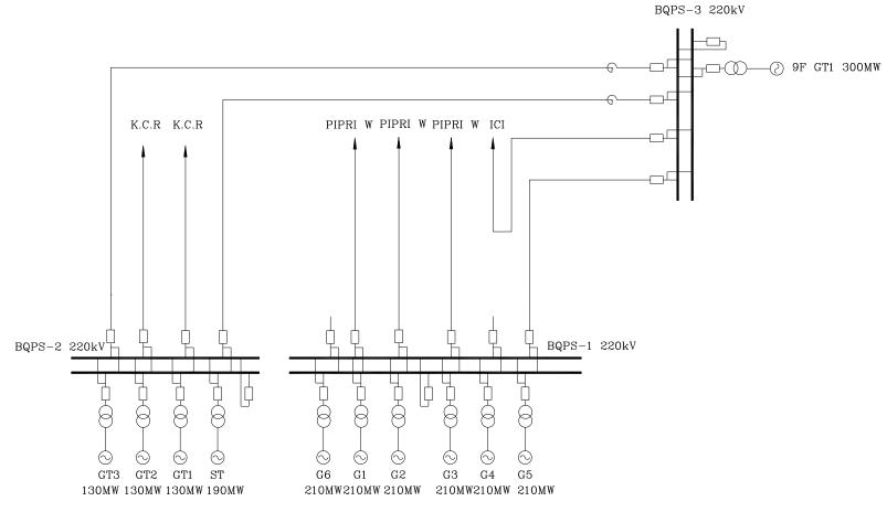
Fig 2.8-1 The SLD of 220 kV GIS with 1<sup>st</sup> 9F Open Cycle in Phase one
