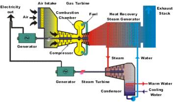
Figure 4: Combined Cycle Turbine System
