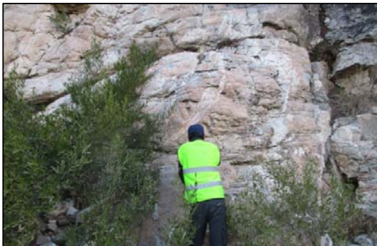
Figure 5.6: Rock outcrop of granite/ granodiorite along the free flow tunnel at discontinuity survey location DS-9.
