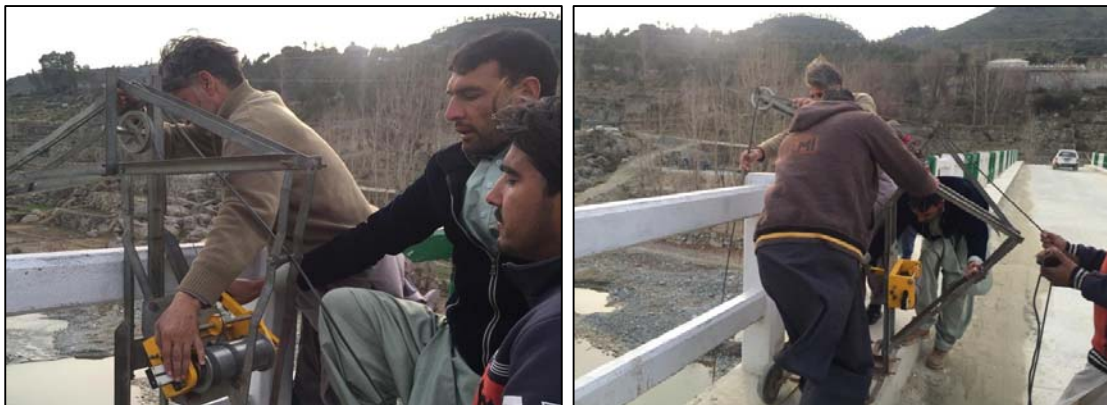
Figure 4-7 Flow Measurements at Artistic- I
