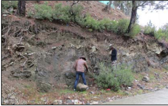
Figure 5.8: Foliated/ Sheared Amphibolite outcrop along the road near cut & cover (or daylight) location at the right bank (DS-3 location) of right bank stream joining Panjkora River.
