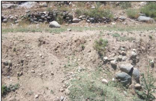
Figure 5.4: Slope wash material at the right abutment of the weir.
