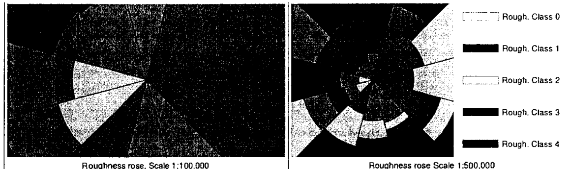
Figure 6-5: Roughness rose for Iran - Pak wind park site in Pakistan in two scales
