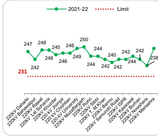
Figure 3.18: Lowest voltage (kV) recorded at 220 kV grid stations under Normal condition
