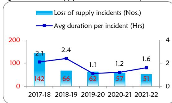
Figure 3.7: Loss of supply incidents along with average
