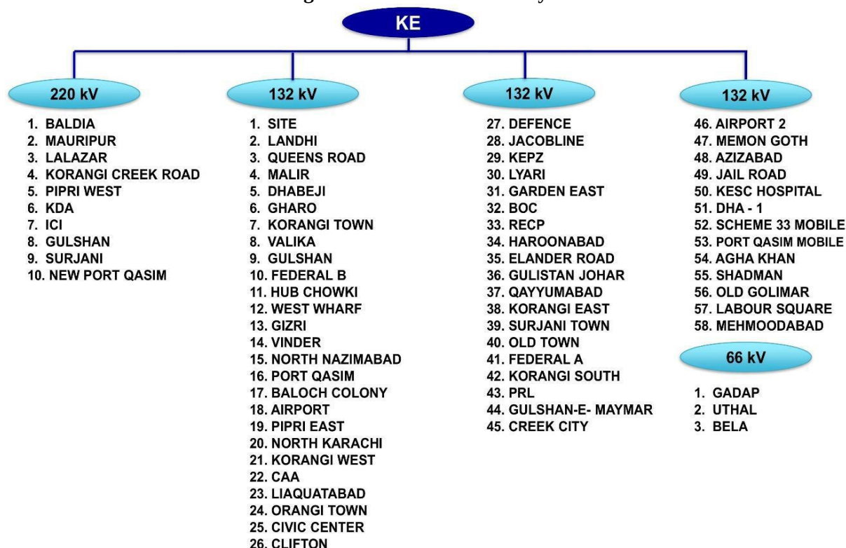
Figure 6.1: KE transmission system
