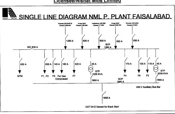
Single line Diagram of the Generation Facility-III/Power Plant-III of the Licensee/Nishat Mills Limited
